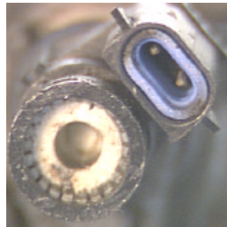
Speed sensor 210 ohms
