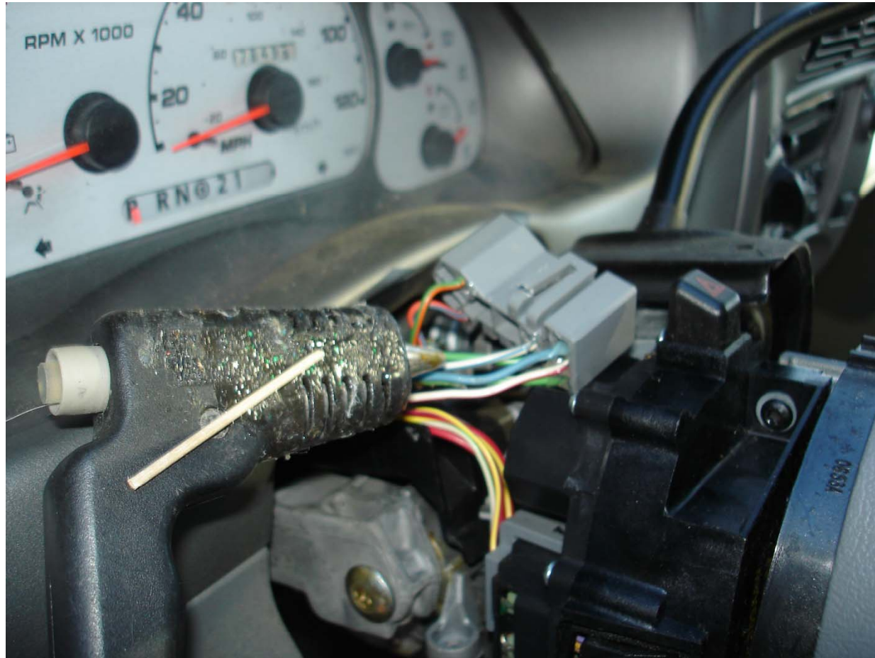
Wires held in place – pushed down in – and hotmelt fed from the back
