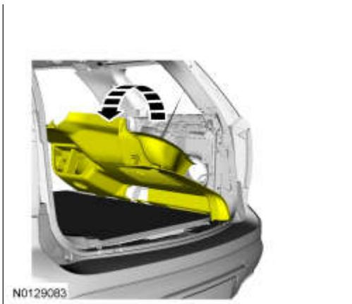
10. Remove the 2 bolts and remove the PAM.
