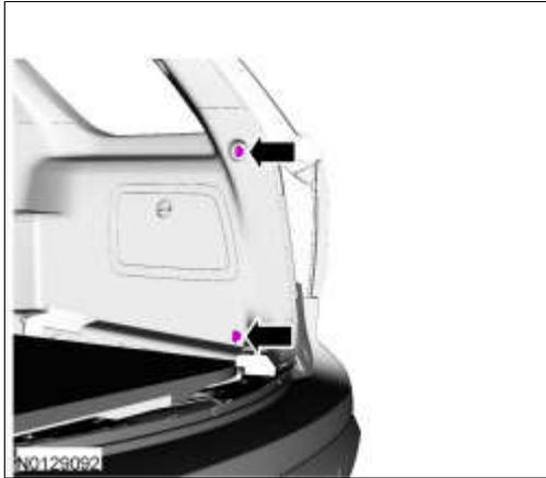
9. **NOTICE:** To avoid damage to the quarter trim panel, remove any retaining clips from the body and attach them to the quarter trim panel before installing.
