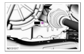
5. *NOTICE:* Use only transmission fluid specific for this transmission. Do not use any supplemental transmission fluid additives or cleaning agents. The use of these products can cause internal transmission components to fail, which will affect the operation of the transmission.
