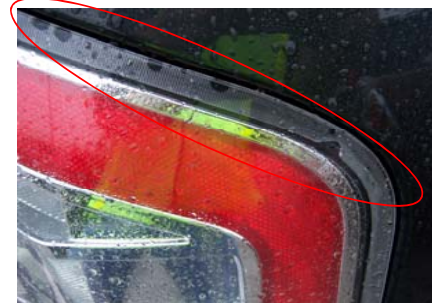
Figure 12: Water droplets outside of lens perimeter.
