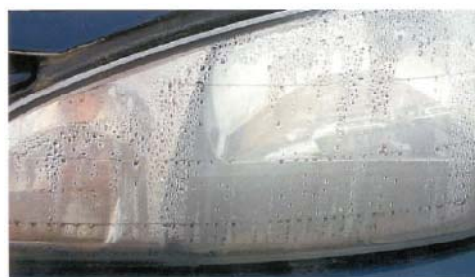
Figure 4: Thick mist covering the lens with water droplets.
