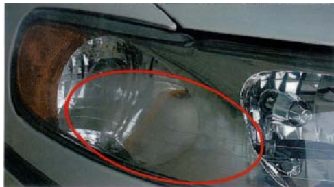
Figure 7: No streaks/ drips marks in the condensation
