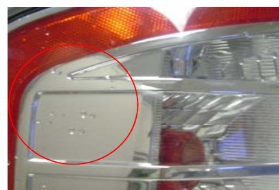
Figure 6: Drip marks/droplets in the interior of lamp
