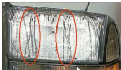
Figure 3: Drip marks/streaks in condensation
