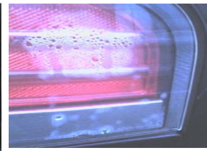
Figure 5: Drips forming in the film condensation
