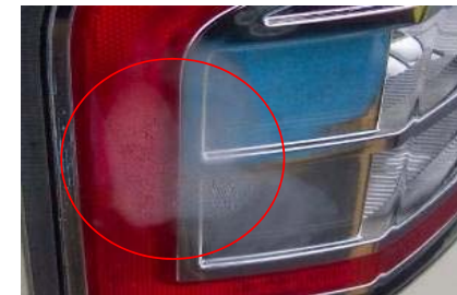
Figure 11: No water droplets in the mist of rearlamps
